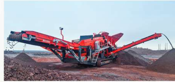
PROVIDES 3 DIFFERENT END-PRODUCTS WITH PRECISE DIMENSIONS BY 2-DECK SCREEN
